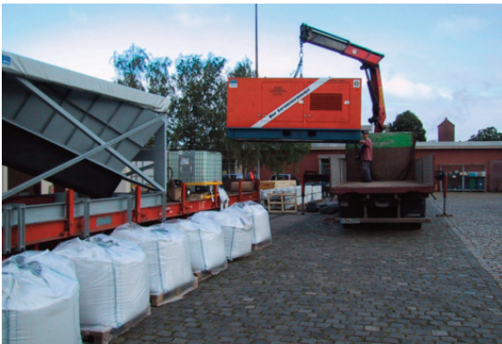
Illustration 7: Upgrading of the DB wagon with conveyor, power set, water tanks and hard and software control systems
