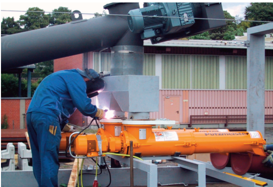
Illustration 9: Installation of the mixer and conveyor on the DB wagon
