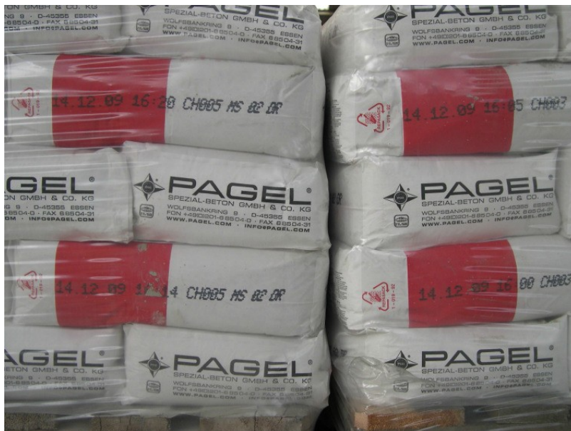
Figure 21: Loading units positioned with tight fit
