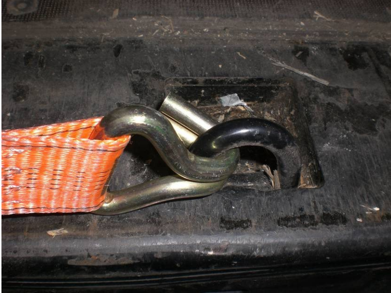
Figure 18: Lashing belt hooked into the lashing point
