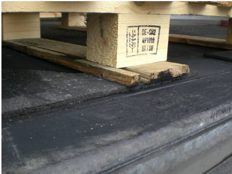
Figure 25: No pallet contact to the vehicle floor
