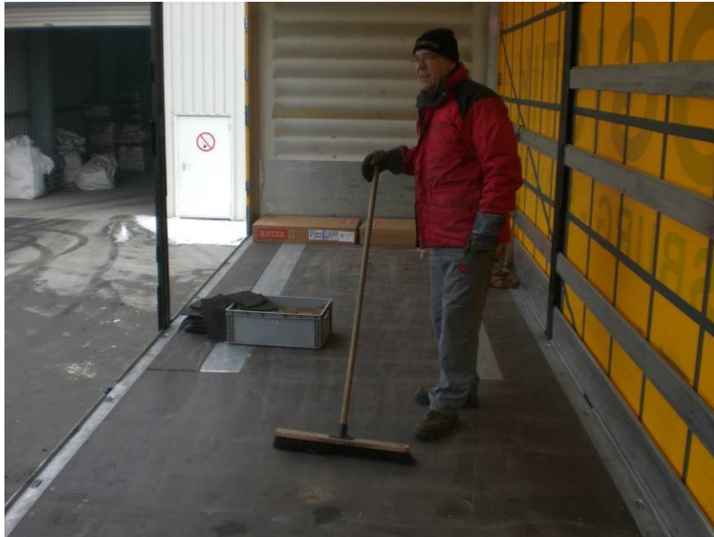
Figure 16: Broom-clean loading area
