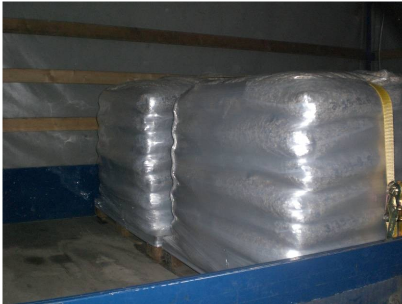
Figure 23: Interposed anti-slip (RH) mats and lashing belt
