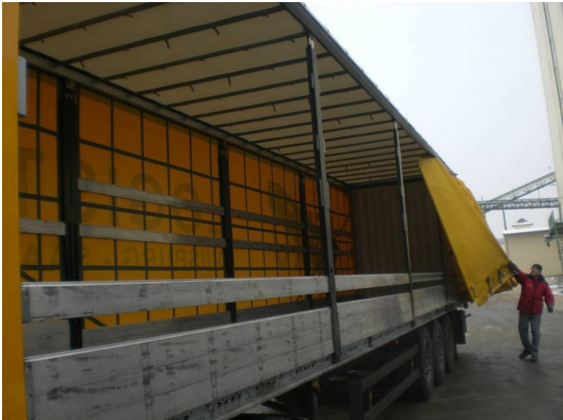
Figure 15: No superstructure parts damaged
