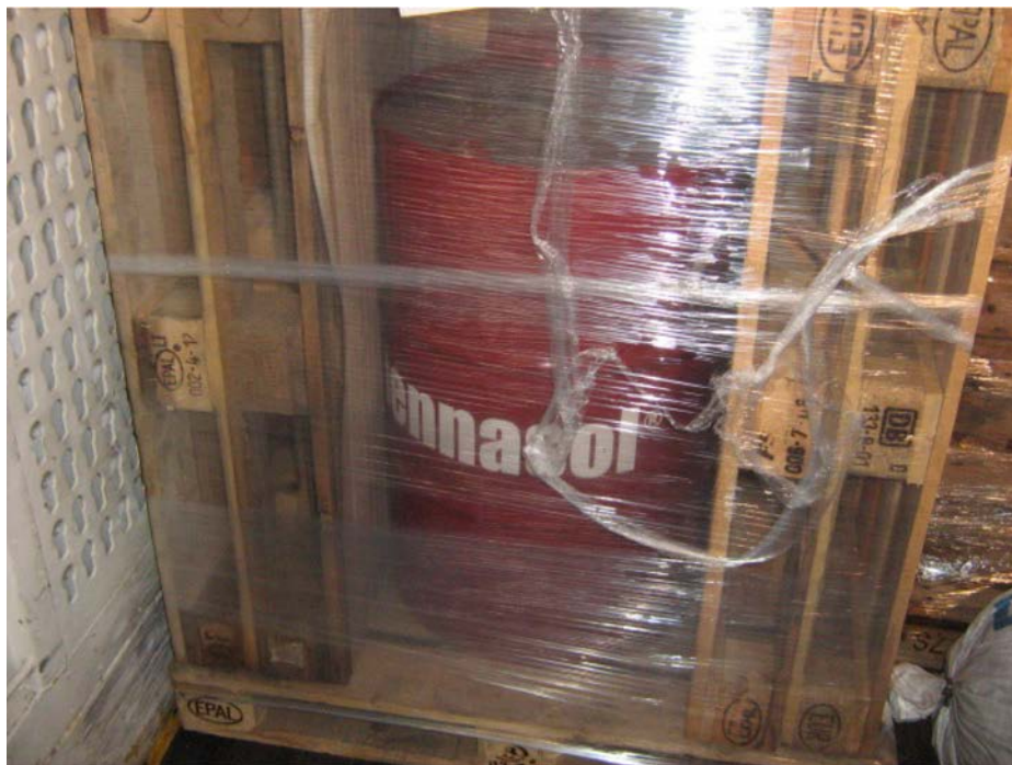
Tight fit by means of additional Euro pallets. How to load individual drums
